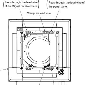
Clamp for lead wire Pass through the lead wire of the i-see Sensor here.
